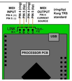
Behind the panel, the LINK bus can also be used to interface with other modules (i.e. ES Disting) and act as a MIDI break-out.
