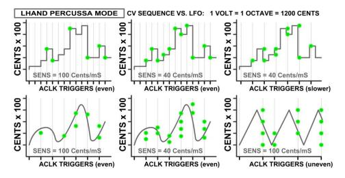
The above image attempts to visually explain Percussa with examples of different Sensitivity levels. The green dots vertically represent number of drums played in a basic way. The ACLK triggers assume LHAND\_T=ACLK1.
