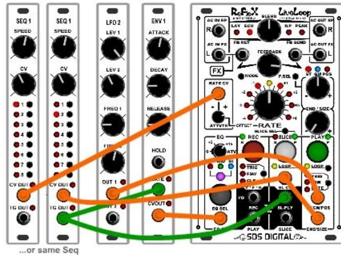
This patch will apply PlayFX mode Start/End to Slices sequencing Globally according to CV inputs for the Start/End controls. Remember the Start/End knobs become + offsets. Position the Start/End knobs as shown in the diagram for this patch. P.SEL ST mode.
