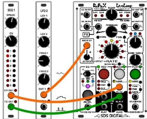
One of the best features of the Reflex LiveLoop is the ability to "address" sample Slices via CV. This method can be used to create a Slice Groove Sequence, where the Reflex plays a recorded sequence on it's own, access sections of a sample in a predictable way to PlayFX them globally, or save a section of a sample to be recalled to start a new Echo from.
