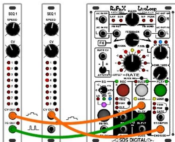
This patch is similar to Patch#4 in that a PlayFX is being used to Globally modify Slices being played, but with G-Move only the first small section of a Slice is played, and the Grain size sets the "note" from a sequencer. Initially the setting for G-Move is GM centered so there is no "move" but adjusted slightly one way or another will allow G-Move to pan the Grain starting anew at every Slice played.
