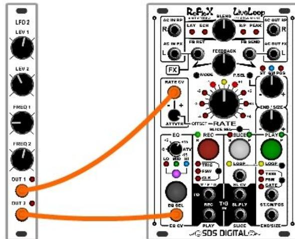
Because both the Rate CV input and the EQ CV input are bipolar, they can both be connected to a +/-5V LFO. The same LFO output can be used for the two, or an inverted output, or second LFO output. Using the two CV inputs together can make a warble in the sample, but with band highlights. This works best when the EQ is on MID or HI or ALL.
