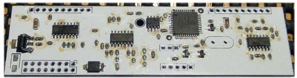
The flux can be cleaned off using alcohol and a toothbrush (that's the problem with white PCB's!)
