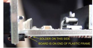
Start with attaching the headers to the panel board, but only the pins on the ends so they can be moved. Flush up the plastic header frame.
