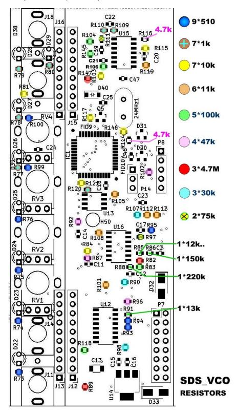
When soldering the small 603 resistors, make a bead on 1 pad for each resistor of the same value, then hold the resistor in place with tweezers (spring closing are best) and move into position over the pad, and perhaps a bit past it to leave the opposite pad exposed some. I count the resistors 1,2,3.. as I'm beading and soldering the second pads.
