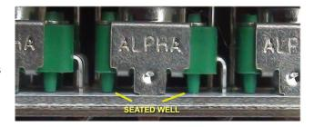
Put all 4 jacks into position. Note that one of the jacks must have it's ground lead bent to reach the hole, so will end up slightly crooked.
