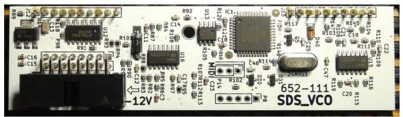
The flux can be cleaned off using alcohol and a toothbrush (that's the problem with white PCB's!) \*Be careful not to get alcohol on the face panel. This may damage the top coat! \*\*BTW P8 (no header) is the programming port. L to R shown: +5V | Gnd | Vpp | PGD | PGC
