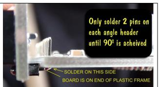
Once 2 pins on each header are soldered, do a test fit. As the final soldering on the main board I would recommend soldering the pins from the back (once panel is on) as some of them come very close to SMD components, but it's up to you!
