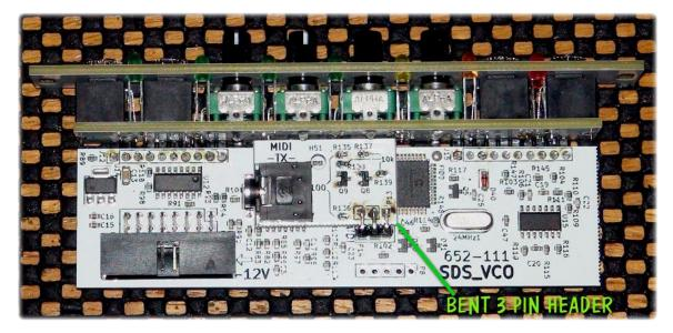
Usin a small plastic clamp will assist in lining up the pins by holding the board. Solder one pin onto the MIDI board first. It can still be moved if needed. Then solder that same pin from the under side of the mother board.
